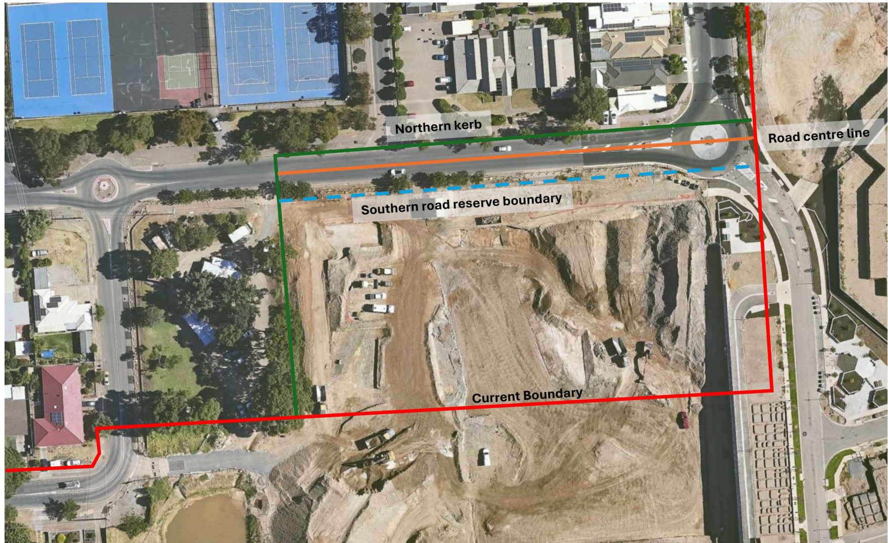
Red = Current Boundary; Orange = Centre line; Blue = Aligns with eventual northern commercial boundary; Green = Northern kerb
